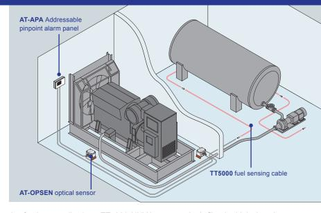
If you have pipes that run externally, there is a specific version for these applications. TT5000-HUV has an synthetic fibre braid designed to wick fuel and provide ultraviolet protection to the sensor. The TT5000 series can also be used in a hazardous area with zener barriers.
