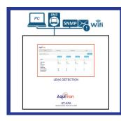
Remote monitoring of the panel via a webserver, easy integration to the buildings IT Network or BMS monitoring.
